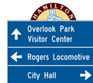
Community Wayfinding Guide Sign with Enhancement Marker
